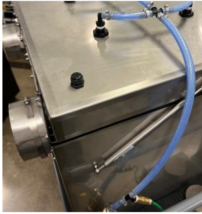
Figure 16: Installed thermocouple port (Black button in corner)
