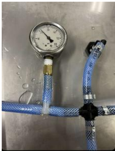
Fig. 18. Pressure Gage 2 Temporarily Installed, Reading the Pressure Before the Nozzles
