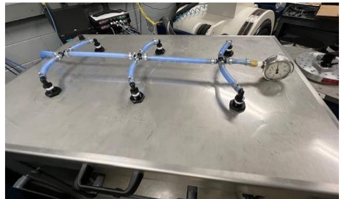
Fig. 15. Hosing layout for dispersing water evenly to each of the 6 nozzles
